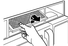
5. Slide a new charcoal filter into place. The filter should rest at the angle shown and set the clock.
