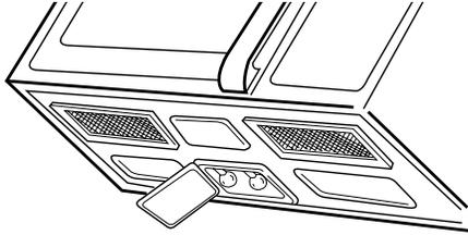
2. Remove the bulb cover mounting screws.
