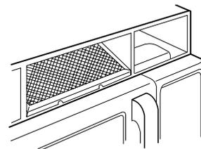
6. Slide the bottom of the vent cover into place. Push the top until it snaps into place. Replace the mounting screws. Turn the power back on at the main power supply and set the clock.
