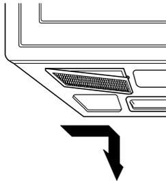
2. Wash in dishwasher or soak grease filters in hot water and a mild detergent. Rinse well and shake to dry. **Do not use ammonia. The aluminum will darken filter.**
