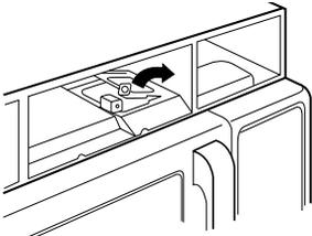
6. Replace bulb with a 30 or 40 watt appliance bulb.
